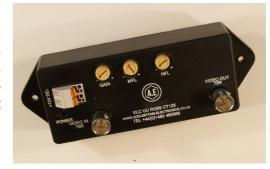
Its installer-friendly design has tool-less adjustable Gain,
